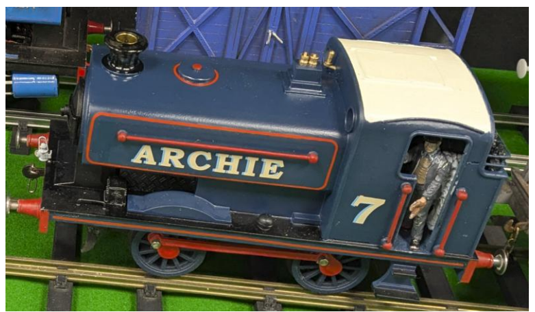
Steve Andrews' weathered NCB loco with added external cylinders, safety valves, bunker and spectacle bars
