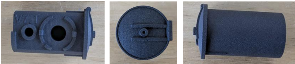
17. Printed black nylon smoke generator and firebox door
