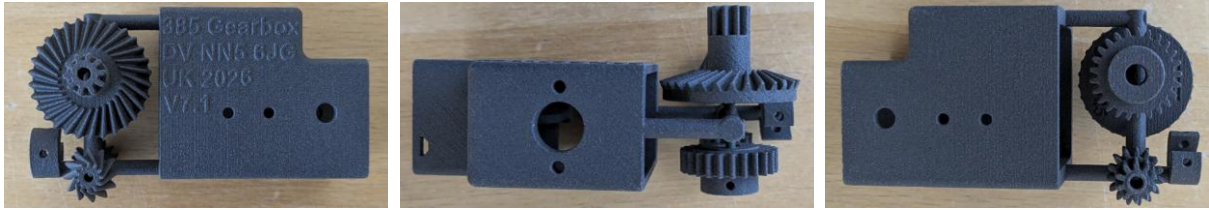
12. Printed nylon sprue with gearbox components
