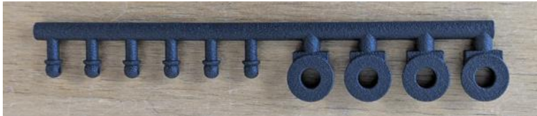
19. Printed nylon sprue with axle boxes and handrail knobs
