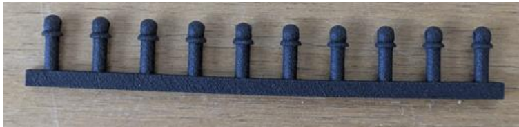
20. Printed nylon sprue with further handrail knobs
