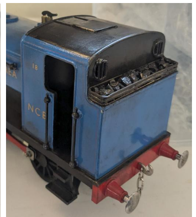
Steve Andrews' weathered NCB loco with added external cylinders, safety valves, bunker and spectacle bars
