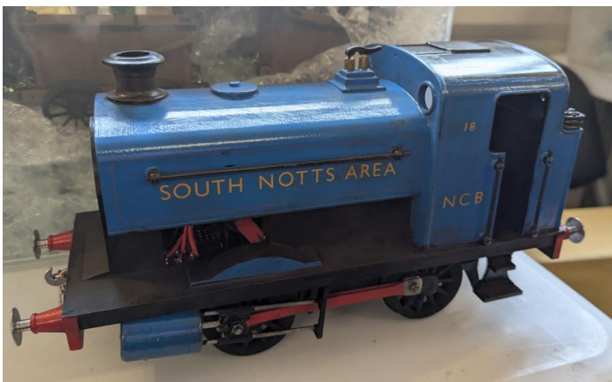
Steve Andrews' weathered NCB loco with added external cylinders, safety valves, bunker and spectacle bars
