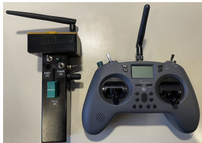
Home-built RC transmitter [L], and miniature transmitter [R].
