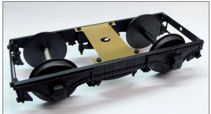
Photo 2: Modified bogie less the central bearing.
