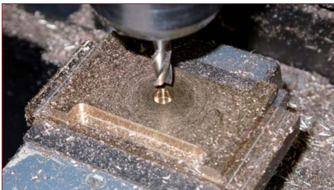
Photo 3: Milling a pack of 10 stretchers in one go.
