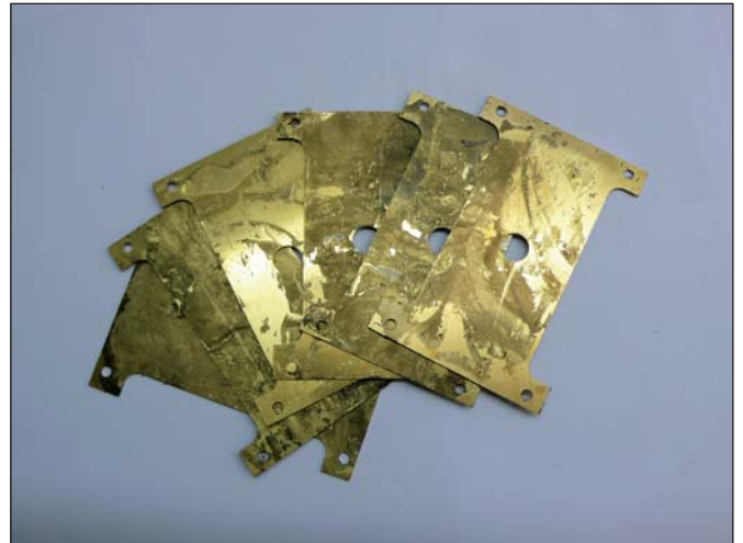
Photo 4: The stretchers, separated after milling and still with glue on them.
