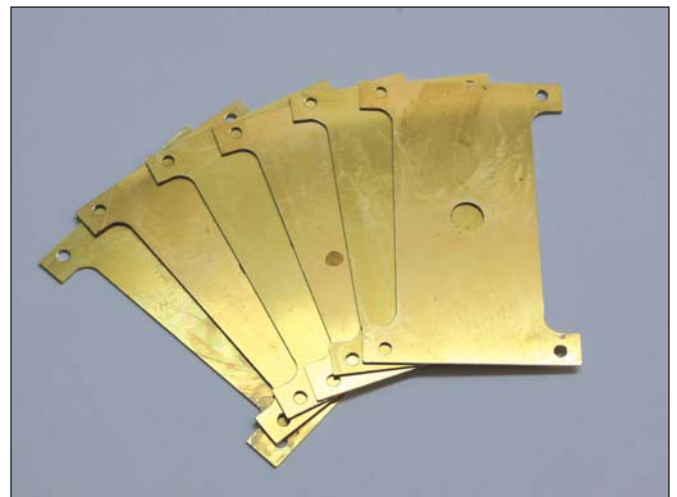
Photo 5: The same stretchers after removing the glue with acetone.
