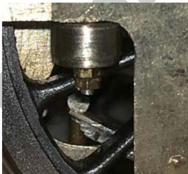
Fig 5-9 a & b Two nuts below spring dampers and close up below
