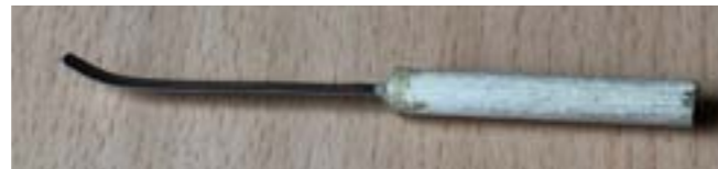
Fig 2-12 Tool to aid removal of bogie wheel set
