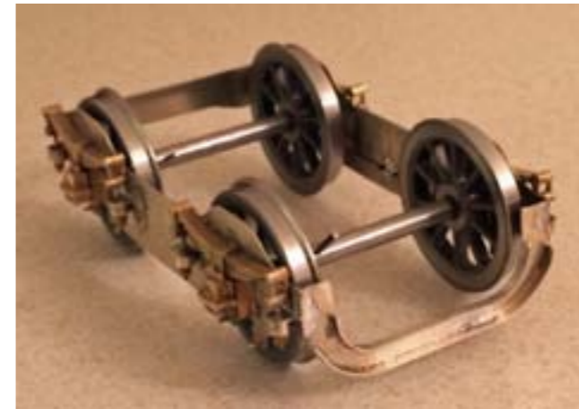
Fig 2-13 Bogie showing U shaped rear stretcher and plainer front stretcher
