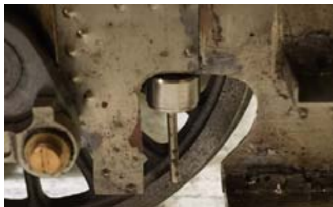
Fig 5-8 Shock absorber fitted but two retaining nuts not yet added
