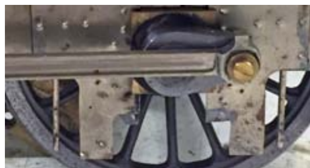
Fig 5-7 The same spring subassembly in position showing the position of rods from spring shackles, dampers not yet fitted at lower ends
