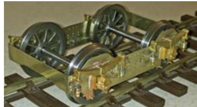
Fig 2-10 Basic assembly up and running with bearings all fitted and temporary stretchers
