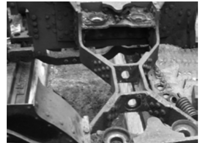
Fig 2-14 Bogie centre arrangement in prototype
