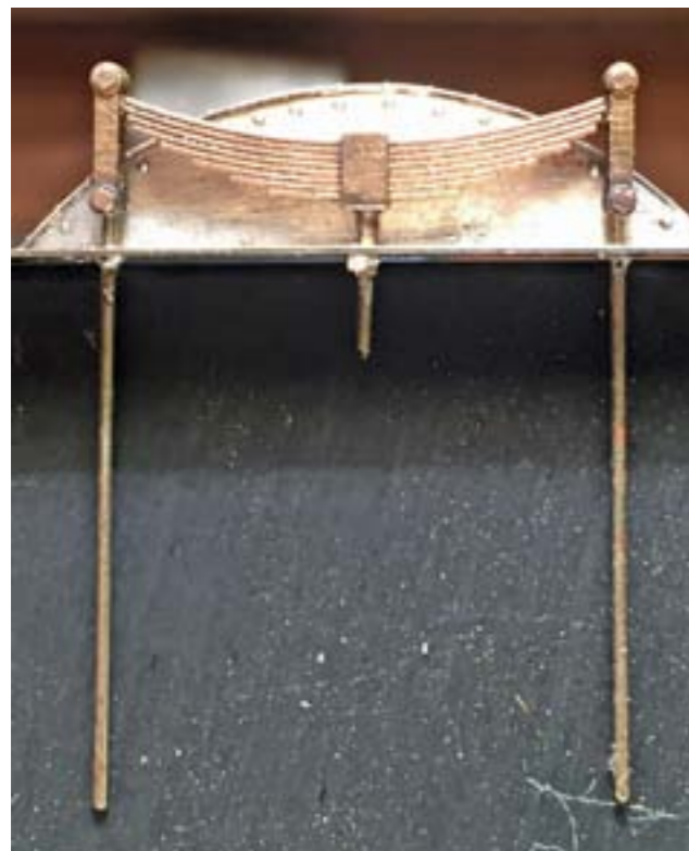
Fig 5-6 Spring subassembly with parts below running plate shown
