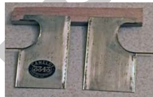
Fig 6-1 Two cab sides not yet finished
