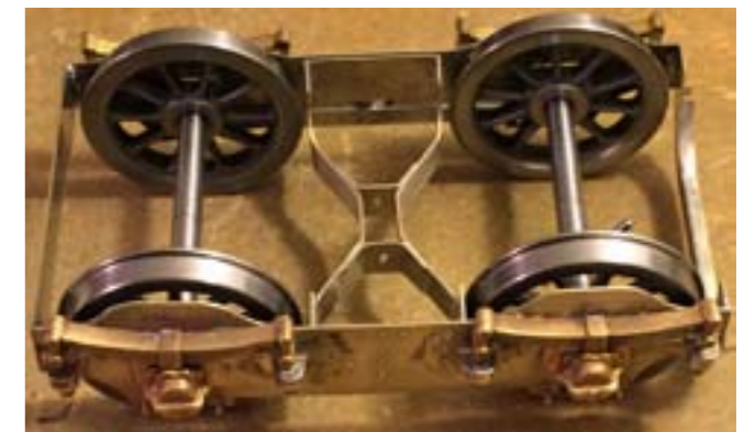
Fig 2-15 Construction of the central cross pieces of the bogie
