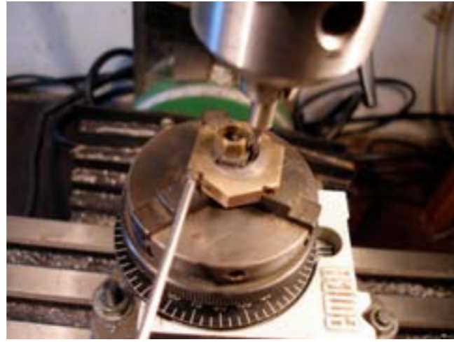
Photo 4.10 Milling the slot
